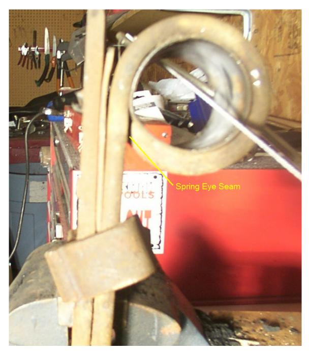
Now thread your hacksaw through the hole, and cut along the spring eye seem until you have cut through the outer bushing.
