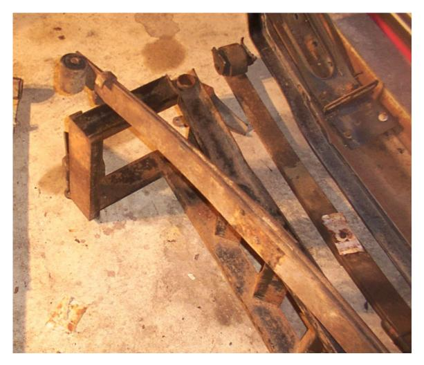
Use a punch or an old spring bolt and nut with a hammer to start the bushing. Remove the center bushing the rest of the way with a pliers.
