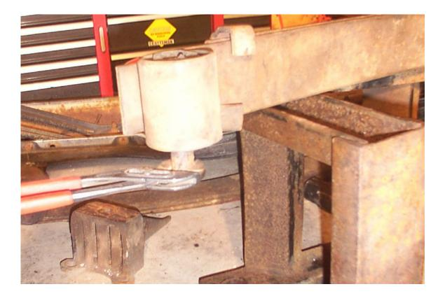
Step 2 – Removing the rubber bushing:
