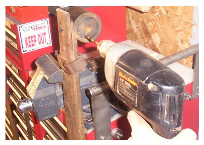
The following picture shows the holes drilled through the bushing. If the holes don't go all the way through the bushing, holes can be drill from the other side.
